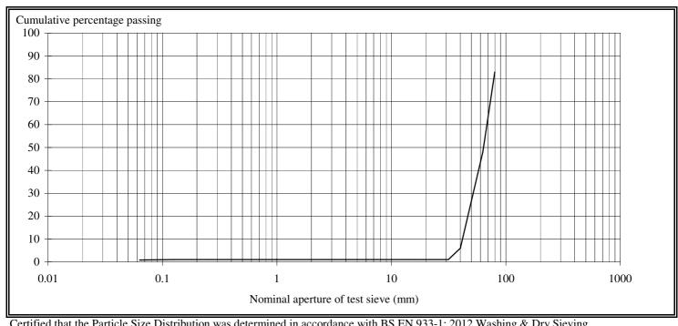
Certified that the Particle Size Distribution was determined in accordance with BS EN 933-1: 2012 Washing & Dry Sieving Certificate of sampling to BS EN 932-1: 1997 received
