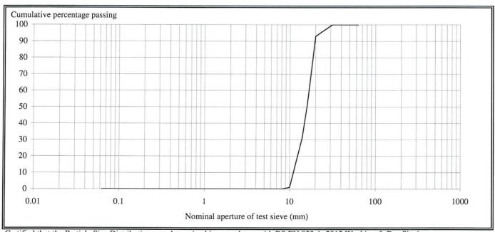
Certified that the Particle Size Distribution was determined in accordance with BS EN 933-1: 2012 Washing & Dry Sieving Certificate of sampling to BS EN 932-1: 1997 not received
